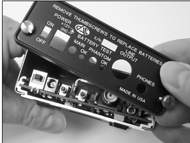
Figure 4: TIP II Rear Panel Removal
